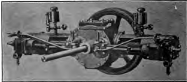
FIG. 24.—Double Opposed Horizontal Cylinder Motor of the Haynes-Apperson Carriages. The two cylinders of this motor are somewhat offset, as shown in the cut, the crank rods working on two cranks. The long crank shaft shown at the front of the engine is for carrying the individual clutch change speed gear. The reciprocating parts are lubricated by adjustable oil feed cups shown at the top of each cylinder. Ignition is by break contact spark, the exhaust connections being on the same plan as those described for other motors. The inlet valves are operated by suction, and are at right angles to the positively operated exhausts.
